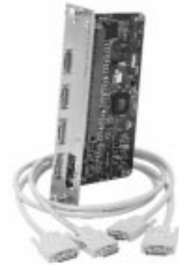
SuperStack II Switch matrix module and SuperStack II Switch matrix cable
