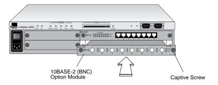
**4** To seat the module, firmly push the module forward to engage the module and backplane connectors. You will feel a slight resistance as the connectors engage.
