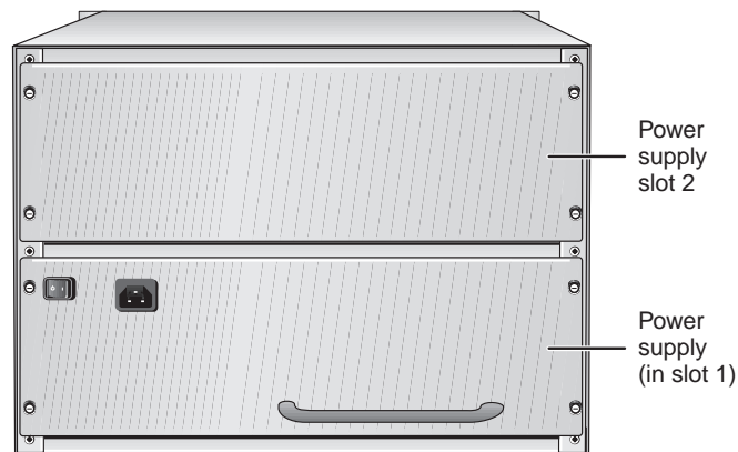
Figure 3 930-watt AC Power Supply in the CoreBuilder 9000 7-slot Chassis
