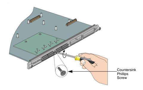
**4** Insert the supplied screws and washers into the daughter card and tighten.
