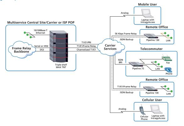
Transport options seamlessly connect remote offices and dial-up users with backbone network services The MAX TNT switch gives users the following options for connecting into a local or remote backbone network:
