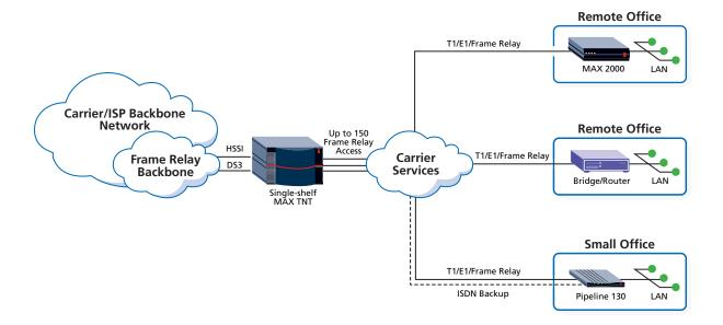
The MAX TNT concentrates up to 150 T1/E1 Frame Relay access lines into a high-speed DS3 network port on the ISP's Frame Relay backbone network. Up to 4094 PVCs per port can be supported.
