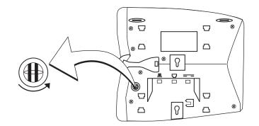
Figure 19 shows an 3Com 2102 Telephone in the wall-mount position. Safe wall mounting requires 3/4-inch drywall and 1.5-inch drywall screws.
