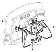
Figure 14 Attaching the Support Bracket
