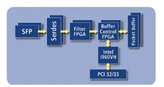
The Xyratex SL1 is a 32 bit / 33 MHz PCI card capable of monitoring two Gigabit Ethernet channels or one full duplex link. It can be attached in-line via taps or at a span port. The Card uses Small Form Factor pluggable MSA compatible optics.
