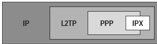
Figure 10. Layer 2 Tunneling Protocol Encapsulation
