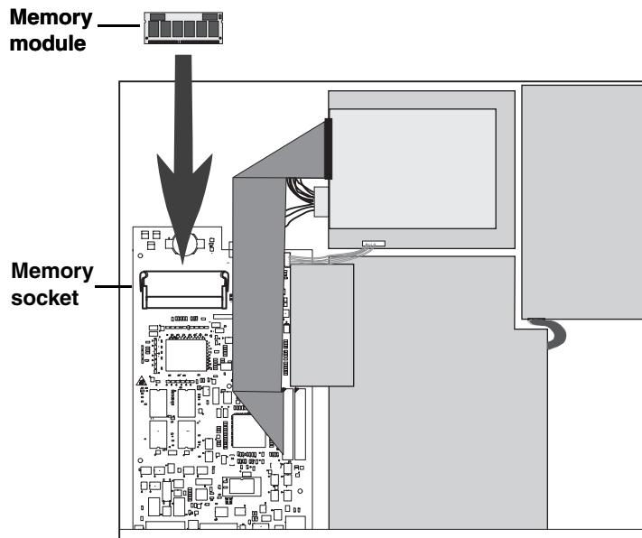
**NOTE:** To remove the memory module, slide both locking tabs away from the memory module until the module pops up, and then remove the memory module from the socket.
