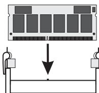
When you insert the memory module, make sure the slot on the module lines up with the tab on the socket.
