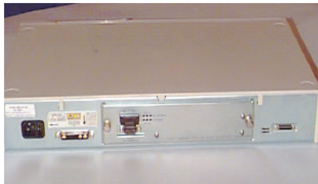
Figure 4 The Installed ATM Expansion Module
