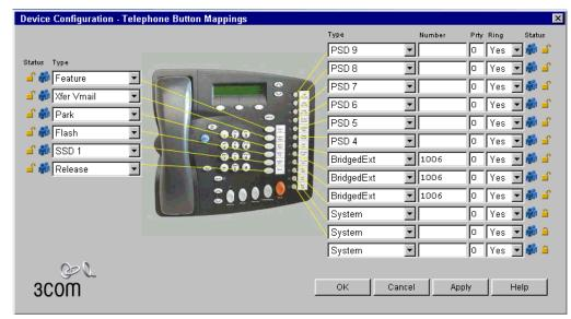
Figure 53 Telephone Button Mappings Dialog Box
